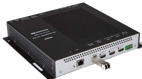
SFP+ Transceiver Module Installation into SFP+ Cage ( DMF-TX-4K-SFP Shown)
